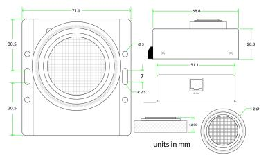
Self calibrating standalone sensor designed for monitoring offgas and H2 in stationary battery systems. Factory calibrated. Self calibrating, no in field calibration required.
