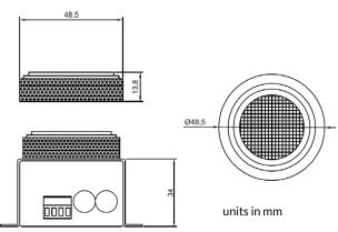
Sensor designed for monitoring flammable gases. User settable address (RS485) out of 256 possibilities. Factory calibrated.
