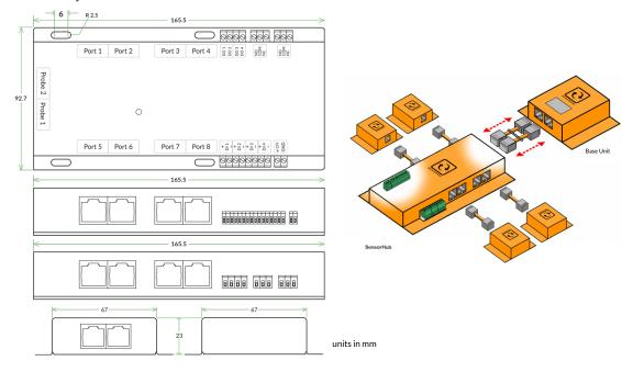
Expands the base unit from 2 to 8 ports & adds control capabilities.
