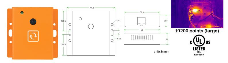
A regular temperature sensor provides you with the temperature of the air surrounding the sensor. The thermal camera sensors provide you with the temperature of the objects & equipment it sees. The world's first SNMP & Modbus thermal camera sensor that tells you the temperature of what it actually sees. 19200 temperature measurement points in one image, analysed every 2 seconds. Minimum and maximum temperature data is available to industrial and IT automation platforms via Modbus TCP or SNMP.
