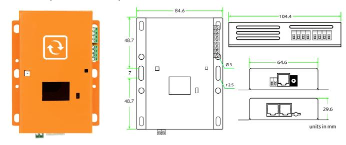
The BASE-SM-6 is an updated version of the Base Unit that includes new built-in features, such as RS485 on a terminal block with 1 relay output. This base unit serves as t he foundational unit for our entire SwitchMon sensor. It boasts a data memory of QSPI 256Mbit and allows for the insertion of an SD Card. Additionally, it has two status LEDs on the PCB.
