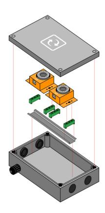
The Environmental Protection Enclosure IP Box is designed to safeguard sensors from outdoor environments. With sufficient airflow, this IP65 rated enclosure allows you to deploy any type of sensor outside, providing protection against weather conditions, falling debris, dust, oil and other non-corrosive materials.
