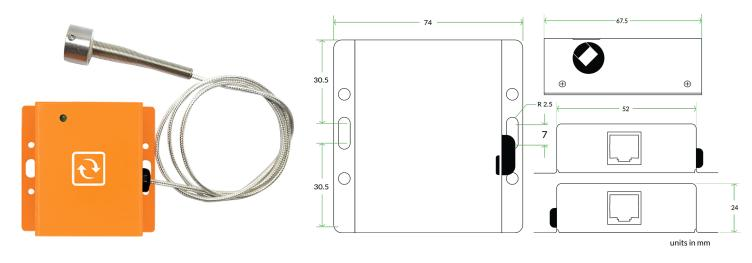
This sensor was designed to monitor temperature in applications where our traditional temperature sensors can't be used. The magnetic probe can be attached to any metal surface and measure its temperature and has a high temperature silver plated shielded wire with strong magnetism and strong absorption.
