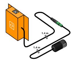
The C-ENV-THUM is a cylindrical version of plug & play sensor designed for monitoring temperature & humidity inside racks and hot/cold aisles in data center white spaces by hanging from ceiling.
