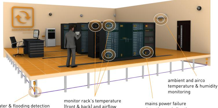
water & flooding detection under raised floors
